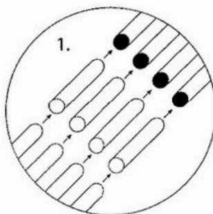
**ENG:** Insert the poles into the plastic connectors.
